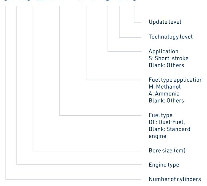
Example engine designation 6X52DF-A-S1.0 representing a WinGD 6 cylinder, short-stroke engine for dual-fuel operation with ammonia and diesel.
