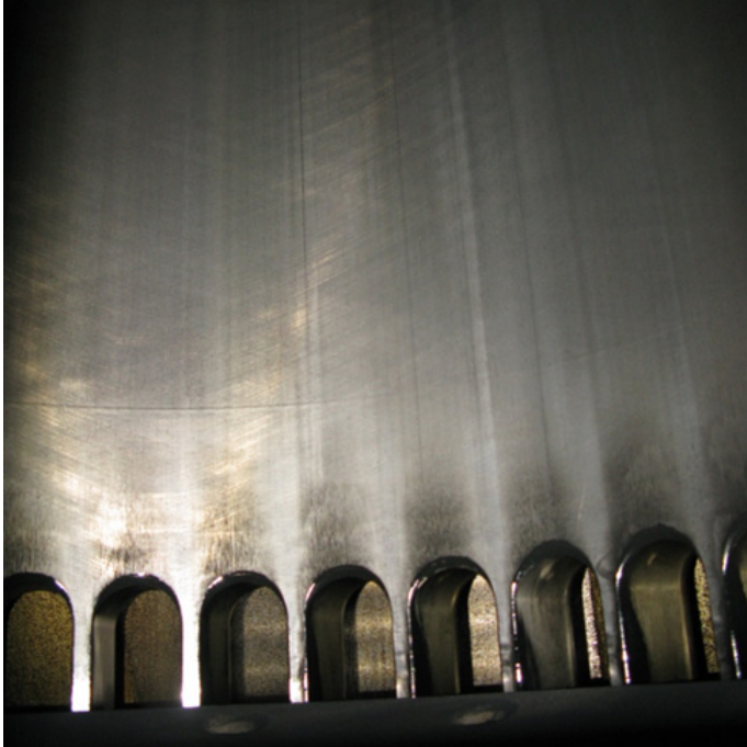
Condition of piston crown top and liner surface above scavenging air port
