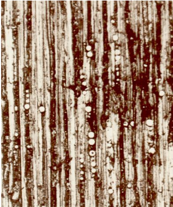
Figure 4. Scuffed cylinder liner surface at TDC with cat fines trapped in graphite flakes.
