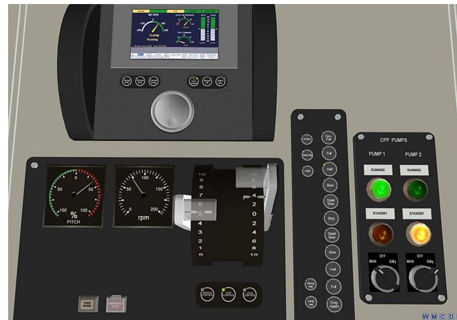
Action screen, example showing close view on the propulsion control system panel selected
