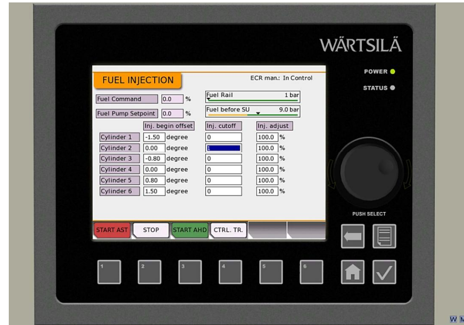
Virtual LDU operator's interface with example adjustments of fuel injection begin offset
